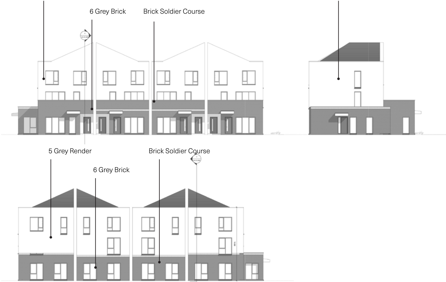
Typical Duplex Elevations
